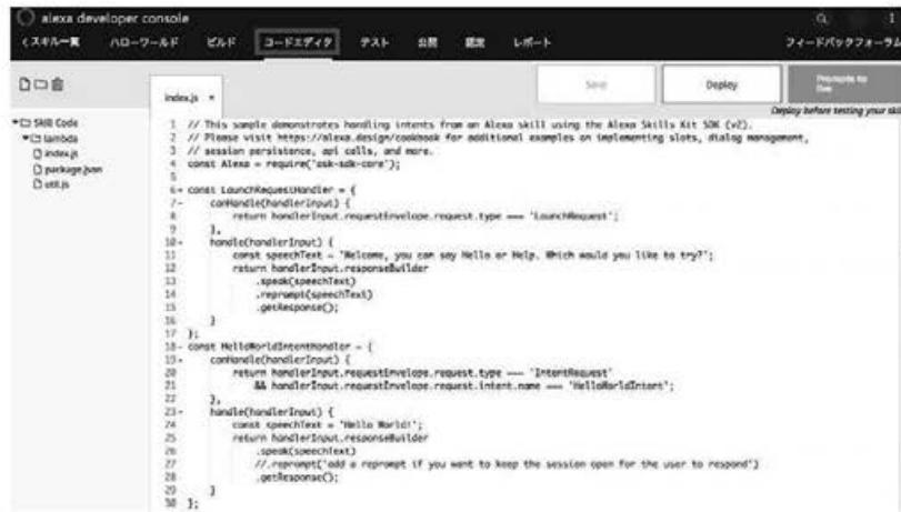
The screenshot shows the Alexa developer console interface. The top navigation bar includes tabs for Skill List, Hello World, Build, Code Editor (which is currently selected), Test, Publish, Settings, and Report. Below the navigation is a toolbar with Save, Deploy, and Deploy before testing your skill. The main area displays the code for index.js:
